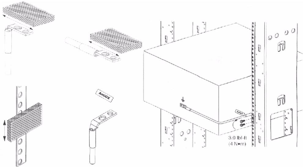
**Figure 10** Equipment Mounting Diagram
