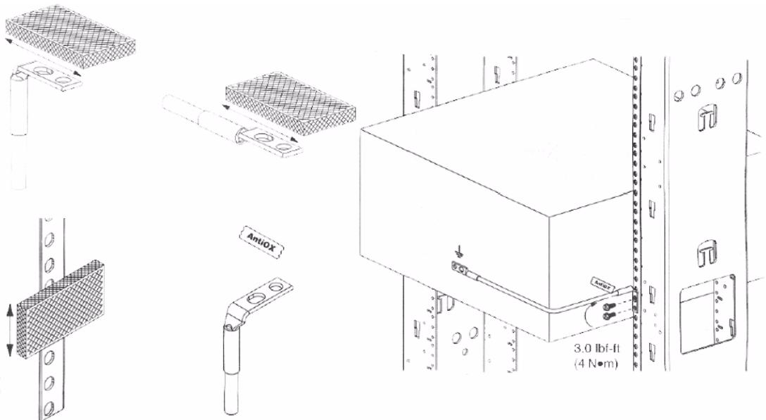
**Figure 4** NEBS Compliant Equipment Mounting Diagram
